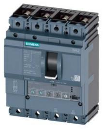
CIRCUIT BREAKER 3VA2 IEC FRAME 100 BREAKING CAPACITY CLASS H ICU=85KA @ 415 V 4POLE, LINE PROTECTION ETU350, LSI, IN=100A OVERLOAD PROTECTION IR=40A ...100A SHORT CIRCUIT PROTECTION ISD=1,5... 10 X IR, II=12 X IN NEUTRAL PROTECTION ADJUSTABLE(OFF,50%,100%) BUSBAR CONNECTION
