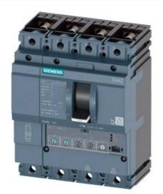
CIRCUIT BREAKER 3VA2 IEC FRAME 160 BREAKING CAPACITY CLASS C ICU=110KA @ 415 V 4POLE, LINE PROTECTION ETU330, LIG, IN=63A OVERLOAD PROTECTION IR=25A ...63A SHORT CIRCUIT PROTECTION II=1,5...12 X IN NEUTRAL PROTECTION ADJUSTABLE(OFF,100%) GROUNDFAULTPROTECTION IG=0,2... 1 X IN, TG=0,1/0,3MS BUSBAR CONNECTION
