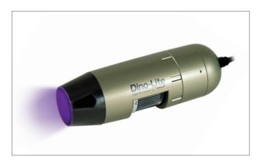
The VW series has two types of LED lights that are switchable between white and UV light. This model has a filter to filter out the returning UV light so that an image with natural colors can be obtained. Also available without return filter (model AM4113T-VW) and in a version with 390-400nm LEDs (model AM4113T-FVW).
