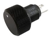
The P16S is a revolutionary concept in panel mounted potentiometers. This unique design consists of a knob driving and incorporating a cermet potentiometer. Only the mounting hardware and terminals are situated on the back side of the panel reducing to a minimum the required clearance.
