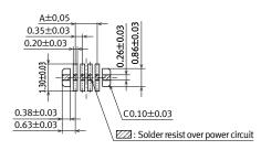
Recommended metal mask pattern Metal mask thickness: When 80 µm (Terminal opening ratio: 50%)
