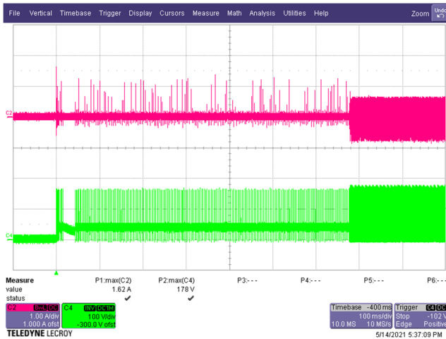
Figure 24 – Primary Clamp Drain Voltage and Current. 90 VAC, 5.0 V, 3 A Load (178 V MAX ). C4: V DRAIN , 100 V / div. C2: I DRAIN , 1 A / div. Time: 100 ms / div.
