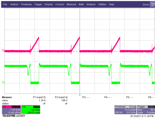
Figure 36 – Primary Drain Voltage and Current. 90 VAC, 5.0 V, 3 A Load (188 V MAX ). C4: V DRAIN , 100 V / div. C2: I DRAIN , 1 A / div. Time: 10 μs / div.
