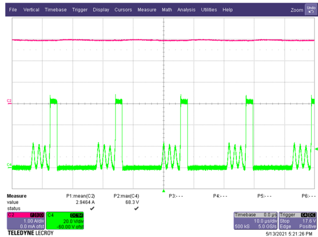
Figure 55 – SR FET Drain Voltage and Current. 265 VAC, 9.0 V, 3 A Load (68.3 V MAX ). C4: V DRAIN(SR) , 20 V / div. C2: I LOAD , 1 A / div. Time: 10 μs / div.
