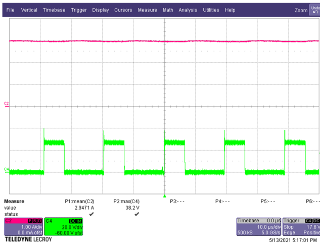
Figure 54 – SR FET Drain Voltage and Current. 90 VAC, 9.0 V, 3 A Load (38.2 V MAX ). C4: V DRAIN(SR) , 20 V / div. C2: I LOAD , 1 A / div. Time: 10 μs / div.
