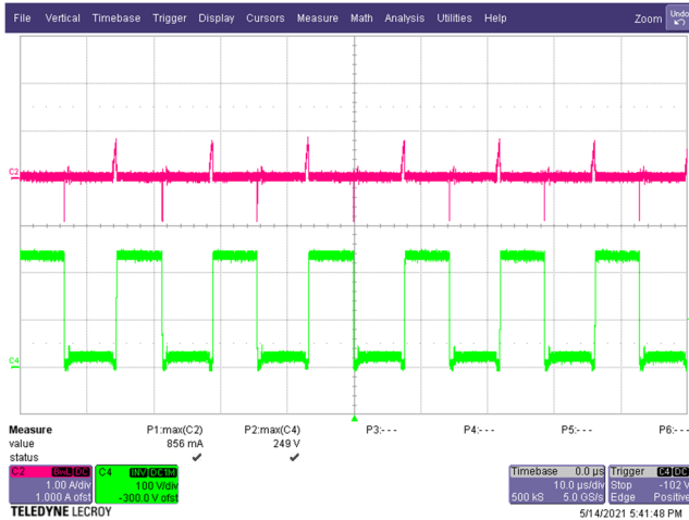
Figure 48 – Primary Clamp Drain Voltage and Current. 90 VAC, 15.0 V, 3 A Load (249 V MAX ). C4: V DRAIN , 100 V / div. C2: I DRAIN , 1 A / div. Time: 10 μs / div.
