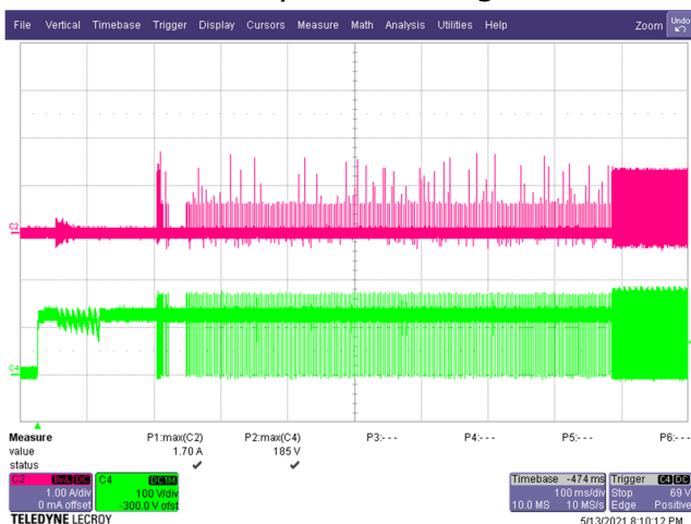
Figure 22 – Primary Drain Voltage and Current. 90 VAC, 5.0 V, 3 A Load (185 V MAX ). C4: V DRAIN , 100 V / div. C2: I DRAIN , 1 A / div. Time: 100 ms / div.
