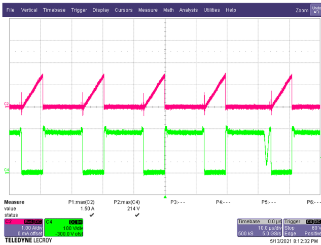
Figure 38 – Primary Drain Voltage and Current. 90 VAC, 9.0 V, 3 A Load (214 V MAX ). C4: V DRAIN , 100 V / div. C2: I DRAIN , 1 A / div. Time: 10 μs / div.
