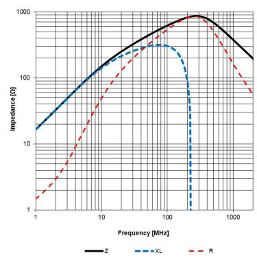
Test Equipment: E4991A or equivalent
