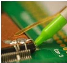
Figure 5. Copper Pad on IC
