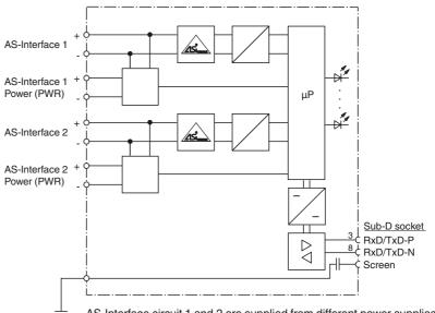
AS-Interface circuit 1 and 2 are supplied from different power supplies. The gateway is supplied from circuit 1. At the cable for power supply no slaves or repeaters may be attached.
