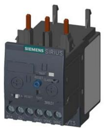
OVERLOAD RELAY 0.1...0.4 A FOR MOTOR PROTECTION SIZE S0, CLASS 5...30 CONTACTOR ASS. MAIN CIRCUIT: SCREW CONN. AUX.CIRCUIT: SCREW CONN. MANUAL-AUTOM.-RESET INT. GROUND FAULT DETECTION
