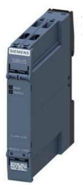
Thermistor motor prot. relay Standard evaluation unit 17.5 mm enclosure Screw terminals 1 NO contact, 1 NC contact US = 24-240 V AC/DC Auto RESET Suitable for bimetal switches 2 LEDs (READY/TRIPPED) Galvanic separation
