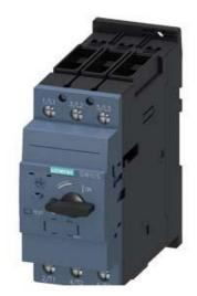
CIRCUIT BREAKER SIZE S2, FOR MOTOR PROTECTION, CLASS 20, A-REL. 22...32A, N-REL. 416A, SCREW TERMINAL, STANDARD BREAKING CAPACITY
