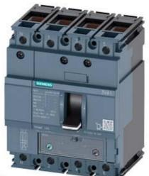
CIRCUIT BREAKER 3VA1 IEC FRAME 160 BREAKING CAPACITY CLASS N ICU=25KA @ 415 V 4-POLE, LINE PROTECTION TM240, ATAM, IN=100A OVERLOAD PROTECTION IR=70A ...100A SHORT CIRCUIT PROTECTION II=5...10 X IN NEUTRAL UNPROTECTED CABLE CONNECTION
