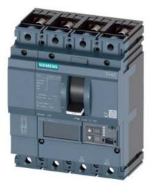
CIRCUIT BREAKER 3VA2 IEC FRAME 160 BREAKING CAPACITY CLASS M ICU=55KA @ 415 V 4POLE, LINE PROTECTION ETU850, LSI, IN=40A OVERLOAD PROTECTION IR=16A ...40A SHORT CIRCUIT PROTECTION ISD=0,6..10X IN, II=1,5..12X IN NEUTRAL PROTECTION ADJUSTABLE (OFF, UPTO 160%) BUSBAR CONNECTION
