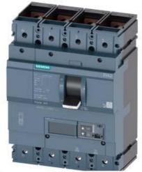
CIRCUIT BREAKER 3VA2 IEC FRAME 400 BREAKING CAPACITY CLASS H ICU=85KA @ 415 V 4-POLE, LINE PROTECTION ETU860, LSIG, IN=250A OVERLOAD PROTECTION IR=100A ...250A SHORT CIRCUIT PROTECTION ISD=0,6..10X IN, II=1,5..12X IN NEUTRAL PROTECTION ADJUSTABLE (OFF, UPTO 160%) GROUND-FAULT, SWITCHABLE IG=0,2... 1 X IN, TG=0,05-0,8MS BUSBAR CONNECTION
