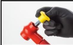
To use the torque wrench for counterclockwise tightening, grip the sliding square from underneath and pull out the sliding square by pressing the lock/unlock button and insert it again on the desired (other) side. Press the lock/unlock button here too.
