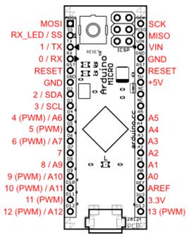
Pin Mapping of the Arduino Micro displays the complete functioning for all the pins, to use them as in the Leonardo.
