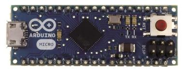
reset button. It contains everything needed to support the microcontroller; simply connect it to a computer with a micro USB cable to get started. It has a form factor that enables it to be easily placed on a breadboard.
