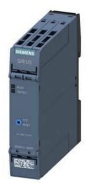
Thermistor motor prot. relay Standard evaluation unit 22.5 mm enclosure Spring-type terminals 2 CO contacts, bistable US = 24-240 V AC/DC Manual/Auto/Remote RESET 2 LEDs (READY/TRIPPED) Galvanic separation Test/Reset button Open-circuit monitoring Short-circuit monitoring Non-volatile
