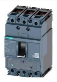
CIRCUIT BREAKER 3VA1 IEC FRAME 160 BREAKING CAPACITY CLASS M ICU=55KA @ 415 V 3-POLE, LINE PROTECTION TM240, ATAM, IN=20A OVERLOAD PROTECTION IR=14A ...20A SHORT CIRCUIT PROTECTION II=5...10 X IN BUSBAR CONNECTION
