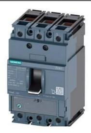
CIRCUIT BREAKER 3VA1 IEC FRAME 160 BREAKING CAPACITY CLASS N ICU=25KA @ 415 V 3-POLE, LINE PROTECTION TM220, ATFM, IN=25A OVERLOAD PROTECTION IR=17,5A ...25A SHORT CIRCUIT PROTECTION II=10 X IN CABLE CONNECTION
