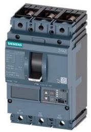
CIRCUIT BREAKER 3VA2 IEC FRAME 160 BREAKING CAPACITY CLASS M ICU=55KA @ 415 V 3POLE, LINE PROTECTION ETU550, LSI, IN=40A OVERLOAD PROTECTION IR=16A ...40A SHORT CIRCUIT PROTECTION ISD=0,6..10X IN, II=1,5..12X IN NEUTRAL PROTECTION OPTIONAL WITH EXT. CT,UPTO 160% BUSBAR CONNECTION
