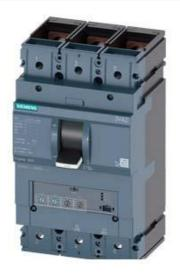
CIRCUIT BREAKER 3VA2 IEC FRAME 400 BREAKING CAPACITY CLASS M ICU=55KA @ 415 V 3-POLE, LINE PROTECTION ETU350, LSI, IN=250A OVERLOAD PROTECTION IR=100A ...250A SHORT CIRCUIT PROTECTION ISD=1,5... 10 X IR, II=12 X IN BUSBAR CONNECTION
