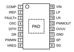
Package LP, 16-Pin eTSSOP Pinout Diagram
