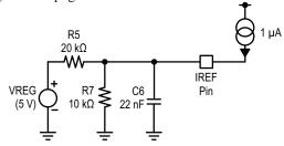
Figure 3: Charging Of Soft-Start Cap During Power Up
