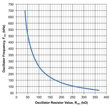
Figure 6: R<sub>OSC</sub> Required for a Particular Oscillator Frequency
