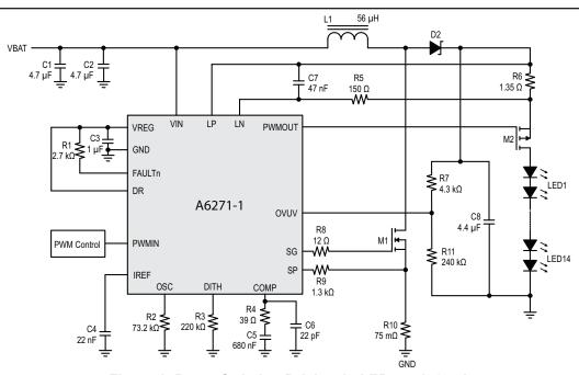
Figure 1: Boost Switcher Driving 14 LEDs at 150 mA
