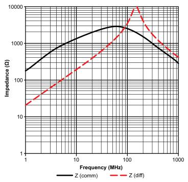
Figure 9: Common-Mode (CM) Choke Impedance
