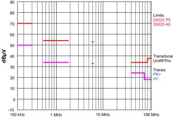
Figure 10: CISPR 25 Class 5 Limit Lines
