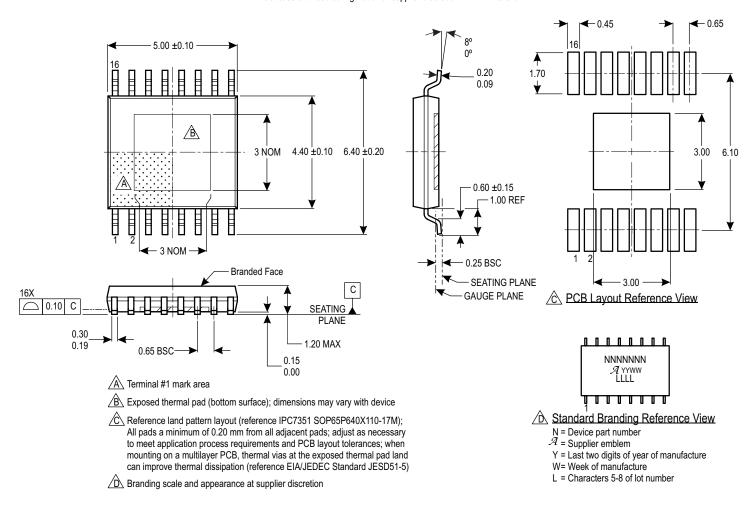
Figure 17: Package LP, 16-Pin eTSSOP with Exposed Thermal Pad
