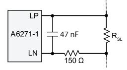
Figure 5: Recommended Current Sensing Network
