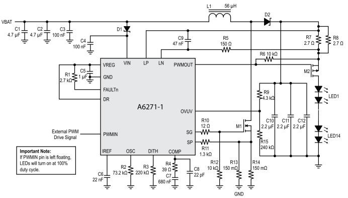
Figure 12: Boost Driving 14 LEDs at 150 mA, Switching Frequency 350 kHz External PWM, no analog dimming, soft-start, and frequency dither on.
