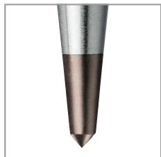
Centre punches made of tool steel are only suitable for work on materials < 40 HRC. For harder materials use centre punches with hard metal tips.
