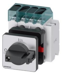
Switch disconnector 3LD3, main switch 3-polig + N, lu 25A operational switch at AC-23 A at 400 V 9,0 kW front mounted Base mounting with center-hole 22,5 mm knob-operated mechanism black  $48 \times 48$  mm with auxiliary 1NO+1NC
