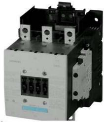
CONTACTOR, 55KW/400V/AC-3 W/O COIL AUXIL. CONTACTS 2NO+2NC 3-POLE, SIZE S6 BAR CONNECTIONS CONVENTIONAL OPERATING MECHAN. AUX.CONDUCTOR: SCREW TERMINALS
