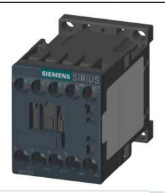
COUPLING RELAY, AC-3, 4KW/400V, 1NO, DC 24V, 0.85...1.85\*US, W. INTEGRATED DIODE 3-POLE SZ S00, SCREW TERMINAL
