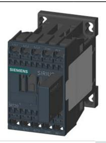
COUPLING RELAY, AC-3, 5.5KW/ 400V 1NC, DC 24V, 0.7...1.25\*US, W. PLUGGED-ON VARISTOR, 3-POLE SZ S00, SPRING-LOADED TERMINAL
