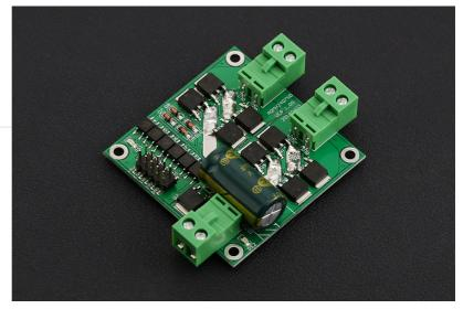
system. It is very considerate to own an Photo Coupler isolation for all the signals in case of that the motor's Reverse Current would interfere the control signals. Besides all, all the interfaces
