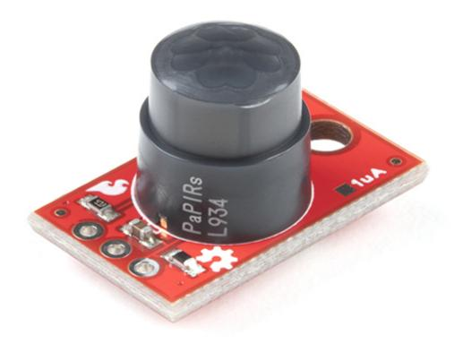
Passive Infrared (PIR) sensors are great for detecting motion in a small area around the sensor. The 170µA SparkFun EKMC4607112K PIR Breakout is a simple board equipped with an EKM-series PIR sensor from Panasonic<sup>®</sup>. The EKM-series PIR sensors are optimized for small movements to offer motion-sensing options for continuously powered applications.
