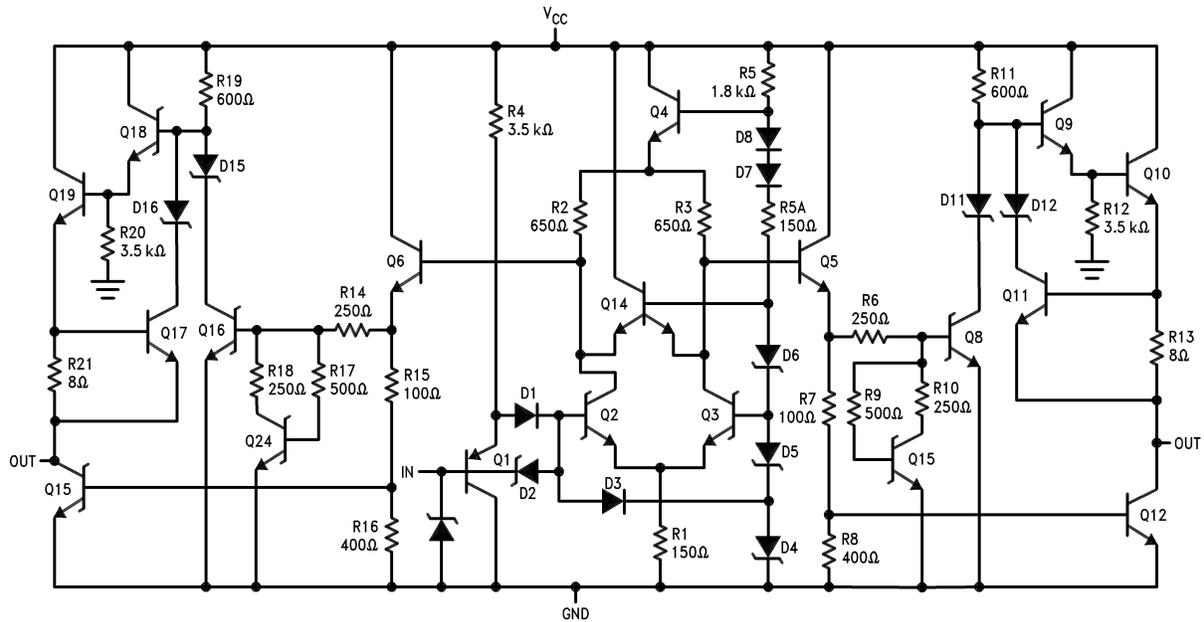
Figure 2. Equivalent Circuit
