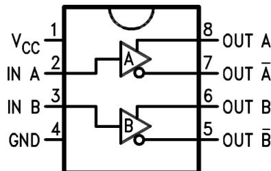
Figure 1. 8-Lead PDIP or CDIP or SOIC (Top View)
