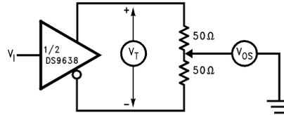
Figure 3. Terminated Output Voltage and Output Balance
