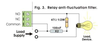
Note: To connect load at 12V DC, you have to remove the resistor and to only use the capacitor.
