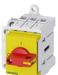
Switch disconnector 3LD3, main switch 3-polig, lu 32A operational switch at AC-23 A at 400 V 11,5 kW Distribution board mounting Base mounting with knob-operated mechanism red/yellow with auxiliary 1NO+1NC
