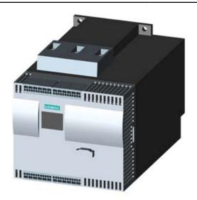
SIRIUS SOFT STARTER, VALUES WITH 575 V, 50 DEG., STANDARD: 32A, 25HP, INSIDE-DELTA CIRCUIT 3: 55A, 50HP, 400-690 V AC, 115 V AC, CAGE CLAMP TERMINALS
