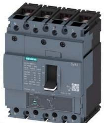
CIRCUIT BREAKER 3VA1 IEC FRAME 160 BREAKING CAPACITY CLASS H ICU=70KA @ 415 V 4-POLE, LINE PROTECTION TM220, ATFM, IN=160A OVERLOAD PROTECTION IR=112A ...160A SHORT CIRCUIT PROTECTION II=10 X IN NEUTRAL PROTECTION 100% BUSBAR CONNECTION
