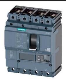
CIRCUIT BREAKER 3VA2 IEC FRAME 160 BREAKING CAPACITY CLASS M ICU=55KA @ 415 V 4POLE, LINE PROTECTION ETU860, LSIG, IN=100A OVERLOAD PROTECTION IR=40A ...100A SHORT CIRCUIT PROTECTION ISD=0,6..10X IN, II=1,5..12X IN NEUTRAL PROTECTION ADJUSTABLE (OFF, UPTO 160%) GROUNDFAULT, SWITCHABLE IG=0,2... 1 X IN, TG=0,050,8MS BUSBAR CONNECTION
