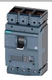
CIRCUIT BREAKER 3VA2 IEC FRAME 400 BREAKING CAPACITY CLASS H ICU=85KA @ 415 V 3-POLE, LINE PROTECTION ETU560, LSIG, IN=400A OVERLOAD PROTECTION IR=160A ...400A SHORT CIRCUIT PROTECTION ISD=0,6..10X IN, II=1,5..10X IN NEUTRAL PROTECTION OPTIONAL WITH EXT. CT;UPTO 160% GROUND-FAULT, SWITCHABLE IG=0,2... 1 X IN, TG=0,05-0,8MS BUSBAR CONNECTION
