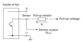
Rated voltage 12 V fan  $V_{CE} = +13.2 V max.$  Ic = 5 mA max. [Vol = Vce (SAT) = 0.6 V max.]
