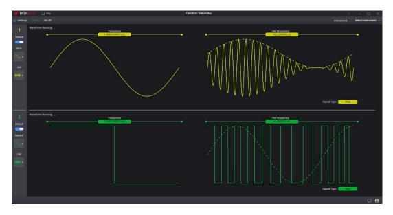
Figure 6. Setting the modulation waveform
