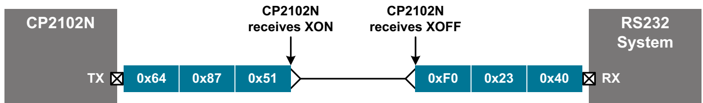
Figure 4.2. Software Flow Control Timing Diagram
