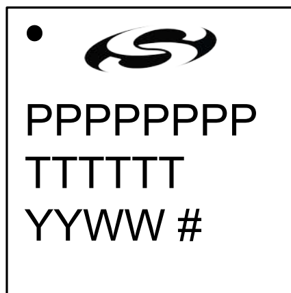
Figure 6.3. QFN28 Package Marking
