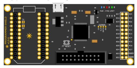
This is a FT2232H based JTAG programmer shield that is compatible with OpenOCD and Broadcom's WICED IDE. The FT2232 chip is setup to provide an USB-JTAG and USB-UART interface simultaneously. The FT2232 can be also reconfigured by the user by reprogramming the on-board configuration EEPROM. The unused pins are clearly marked and broken out into easy to access header holes.
