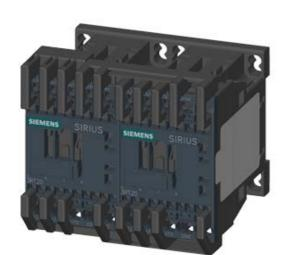
REV. COMB., AC3, 7.5KW/ 400V AC24V, 50/60HZ, 3-POLE, SZ S00 SPRING-LOADED TERMINAL ELECTR. AND MECH. INTERLOCK
