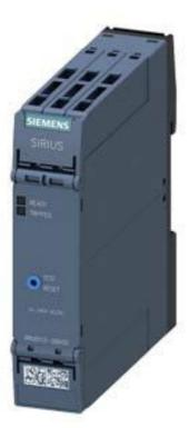
Thermistor motor prot. relay Standard evaluation unit 22.5 mm enclosure Spring-type terminals 2 CO contacts US = 24 V-240 V AC/DC Manual/Auto/Remote RESET with ATEX certification 2 LEDs (READY/TRIPPED) Galvanic separation Test/Reset button Open-circuit monitoring Short-circuit monitoring Non-volatile
