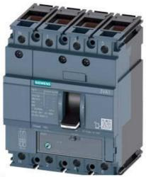
CIRCUIT BREAKER 3VA1 IEC FRAME 160 BREAKING CAPACITY CLASS H ICU=70KA @ 415 V 4-POLE, LINE PROTECTION TM220, ATFM, IN=125A OVERLOAD PROTECTION IR=87,5A ...125A SHORT CIRCUIT PROTECTION II=10 X IN NEUTRAL PROTECTION 100% CABLE CONNECTION
