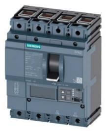
CIRCUIT BREAKER 3VA2 IEC FRAME 160 BREAKING CAPACITY CLASS H ICU=85KA @ 415 V 4POLE, LINE PROTECTION ETU550, LSI, IN=63A OVERLOAD PROTECTION IR=25A ...63A SHORT CIRCUIT PROTECTION ISD=0,6..10X IN, II=1,5..12X IN NEUTRAL PROTECTION ADJUSTABLE (OFF, UPTO 160%) CABLE CONNECTION
