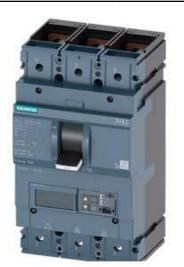
CIRCUIT BREAKER 3VA2 IEC FRAME 630 BREAKING CAPACITY CLASS M ICU=55KA @ 415 V 3-POLE, LINE PROTECTION ETU860, LSIG, IN=500A OVERLOAD PROTECTION IR=200A ...500A SHORT CIRCUIT PROTECTION ISD=0,6..10X IN, II=1,5..14X IN NEUTRAL PROTECTION OPTIONAL WITH EXT. CT;UPTO 160% GROUND-FAULT, SWITCHABLE IG=0,2... 1 X IN, TG=0,05-0,8MS BUSBAR CONNECTION
