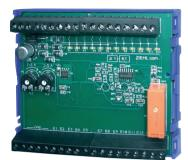
The current relay STW12 monitors the current flow yes/no of up to 12 alternating-current circuits. If there is an AC-current of ≥1 A through a connected transformer STWA 1, the according output transistor switches and the yellow LED lights up.
