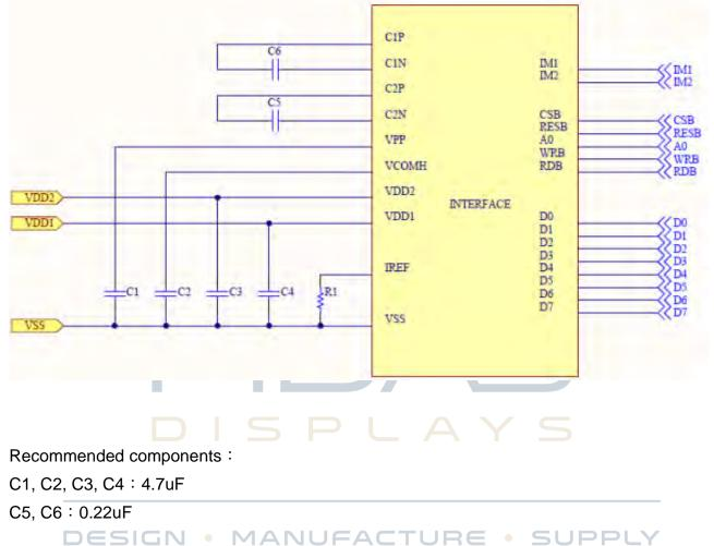
Bus Interface selection: (Must be set the IM[2:0], refer to item 3) 8-bits 6800 and 8080 parallel, 3 or 4-wire SPI, I2C
