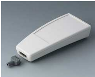
A9068127 SMART-CASE XL, Ausf. III ABS (UL 94 HB) grauweiß RAL 9002 168x74,4x35,4mm IP 65 opt., IP 40
