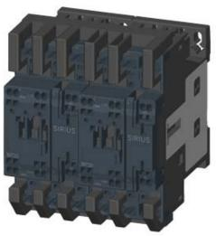
REV. COMB., AC3, 18.5KW/ 400V AC110V 50HZ/120V 60HZ 3-POLE, SZ S0 SPRING-LOADED TERMINAL ELECTR. AND MECH. INTERLOCK 2NO INTEGR.
